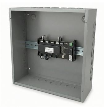
Pre-assembled indoor panel enclosure for Ethernet-to-DMX protocol conversion. Features an 8-port DMX/RDM gateway mounted in a NEMA 1 rated steel enclosure. Converts network-based lighting protocols (sACN, Art-Net) to eight individually configurable DMX512 output ports. Power-over-Ethernet powered for simplified installation with no local power supply required. BAA and BABA compliant for government projects.
